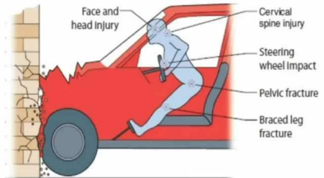
Figure 9.1 Major points of injury to an unrestrained driver of a vehicle in deceleration impact.
